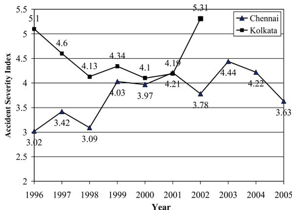
Fig. 1. Accident severity index (persons killed per 100 accidents)
